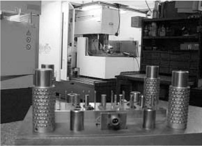
Fig. 3: The bottom half of the progressive die with the "creator" of the punches and dies in the background, an Agiecut Challenge 3.
