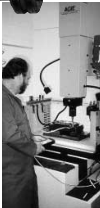
Fig. 4: The setting up of the workpieces on the Agiecut Challenge 3 is made conveniently by manual operation and the workpiece position in the level is automatically plotted with Agiesetup 2D so that there is no longer any need for fine adjustment.
