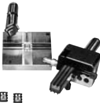
Fig. 4: The setting up of the workpieces on the Agiecut Challenge 3 is made conveniently by manual operation and the workpiece position in the level is automatically plotted with Agiesetup 2D so that there is no longer any need for fine adjustment.
