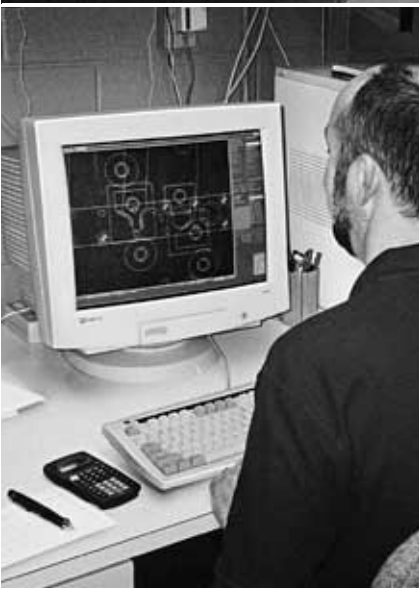
Fig. 2: The workshop drawings for the progressive die for electromechanical contacts which are supplied extrusion-coated to the automotive industry. The geometry programs for EDM are prepared with Peps from Camtek. The CAD program Esprit X is used for the 3D programming of the injection mold.
